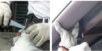
back blade can be used for deburring contour line tapered blade for cutting in small spaces
